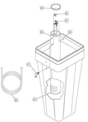
ASSEMBLE THE BRINE TANK: Install a brine well cap (Item A) on the bottom of the brine well (Item B). Remove the brine valve assembly (Item C) from the brine well by removing the nut (Item D). Attach the brine well to the brine tank with the two-piece overflow (Items E & F) using the lower holes in both pieces, as shown. Reinstall the brine valve assembly. Push brine line polytube (Item G) through the upper holes in the brine tank and brine well and press the polytube into the elbow fitting.
