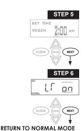
STEP 5 – Next Regeneration Time (minutes): Set the minutes of day for regeneration using or buttons. Press NEXT to return to normal operation. Press REGEN to return to previous step.
